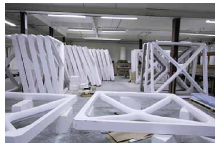
SMIT PLASTICS IN ALKMAAR HAS MANUFACTURED CROSS-SHAPED RIBS MADE OF POLYESTER COMPOSITE WITH A FOAM CORE.
